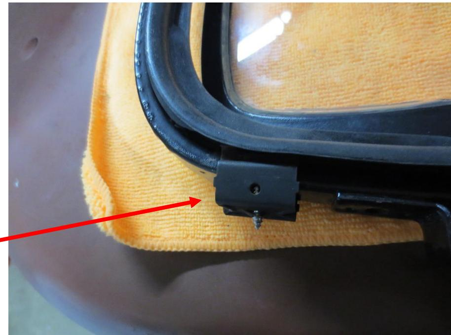
14. Roll the ventilator wing back in place and secure it with screws. Check the weatherstrip to ensure it fits properly on door frame.
