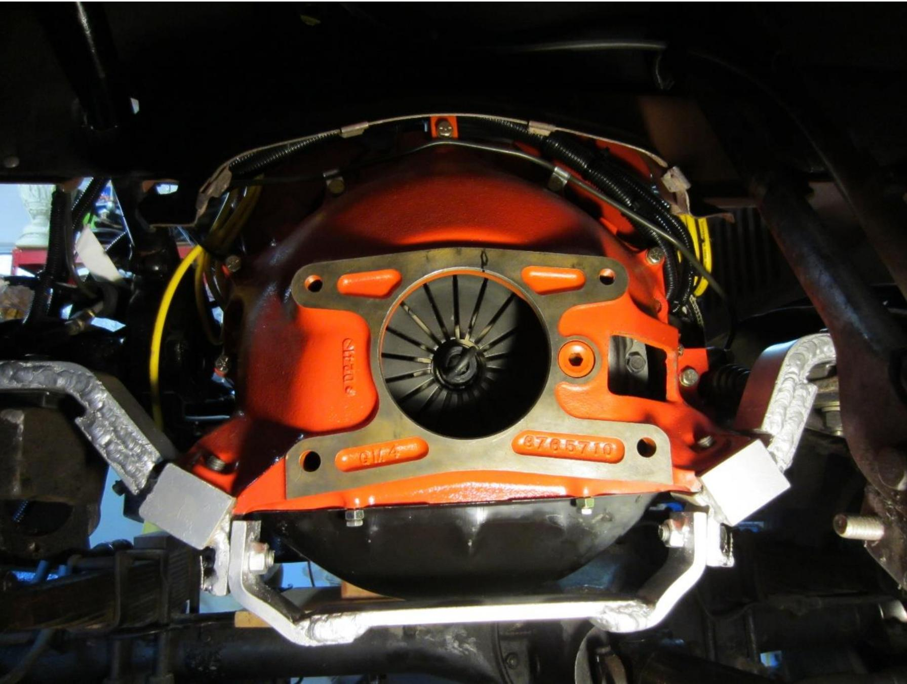
**Set engine on blocks and lever it to the carb mount both ways, side/front. Set the engine  $\frac{3}{4}$ " between distributor and cowl, then begin making the engine mounts, see next image.**
