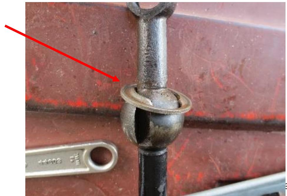
11. Next, install the spring turning it clockwise until the spring is under all the lugs in the housing. Make sure friction plate flange is properly seated in spring and continue installing spring. You will need to use screwdrivers to help work the spring under the last lug.
