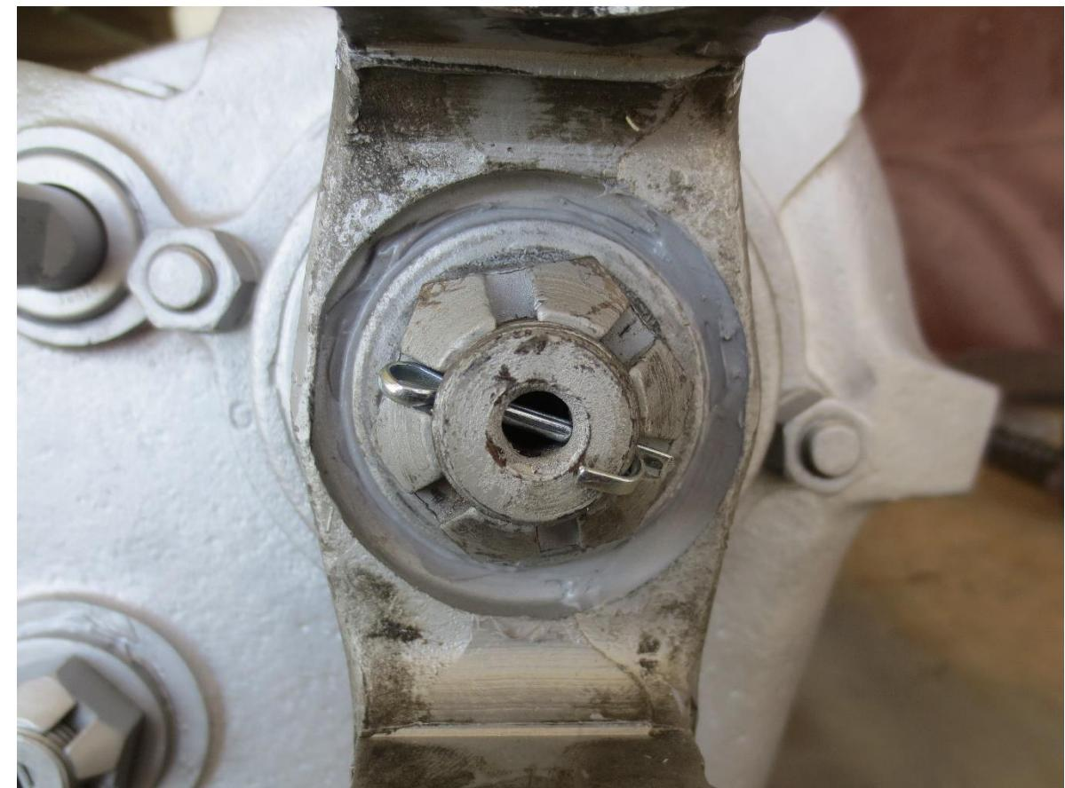
It is important that these studs are in place, they are used to align and provide proper clearance between the idler and driven gears, **DO NOT USE BOLTS**. If bad or missing, stud (C-113247, NSN-5307-00-011-3247) is available in a kit from Oshkosh Equipment Sales [Part Source](#). Use a thread sealer when installing.
