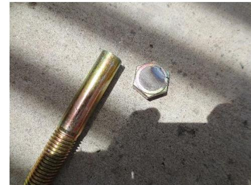
2. Measure to the old shaft and ensure the length of the shaft is long enough to accommodate the lever bushings. Use a shaft collar as a guide to cut consistent grooves around the shaft.
