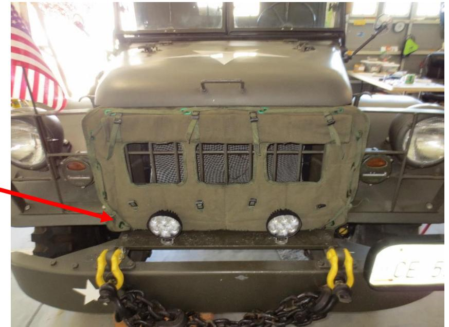
4. Next attached the left retaining spring to the left hole of the cross member, and the right retaining spring to the right crossmember hole. Installation is now complete.
