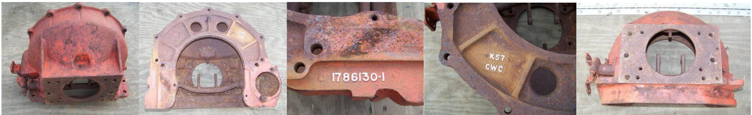
Hemi Engines – 1951-55, 315 C.I.D., 331 C.I.D. casting number 1323329, 1956, 354 C.I.D casting numbers 1551629/1619629, 1957-58, 392 C.I.D. casting number 1619829. Look for 392 blocks with foundry-ID A1, supposedly they have consistently thicker cylinder walls and may have been cast with higher nickel content. A1 is cast in several places, including in the rear face as shown here. How to example for clutch and rear brake master cylinder setup. - [Clutch Setup](#)
