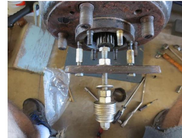
**Pinion Oil Seal Puller** - Pulls front and rear seals. Use a 21/64 drill, then tap holes using 3/8-24 tap. Tighten bolts in seal before pulling.
