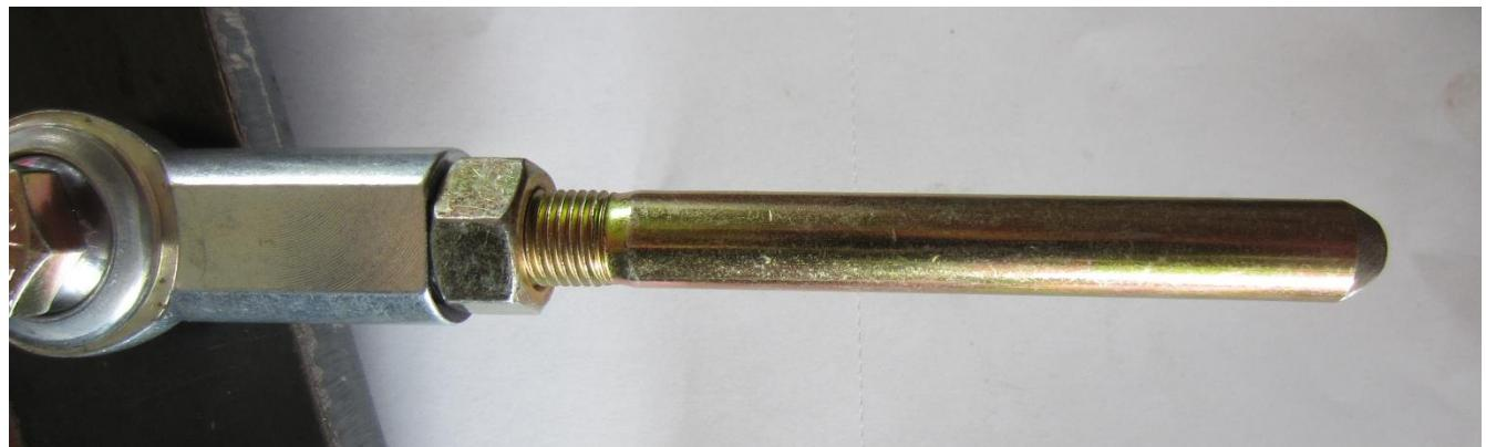
**A bolt is provided for the clutch rod, cut the head off and round the end.**
