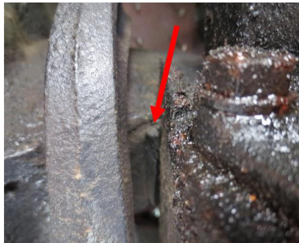
Clearance between the PTO and brake frame mount, transmission 38711 or 1951 to 1956 PW, it needs clearance between those parts.
