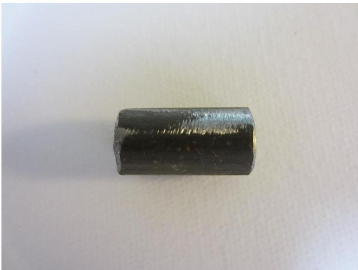
You get three spacers for the Clutch MC in the kit. Only problem is, they are for a  $\frac{1}{4}$ " bolt instead of the  $\frac{5}{16}$ " bolts that are in the kit. You'll need to cut or buy correct new spacers.  $\frac{3}{4}$  is too long the clutch MC will hit the booster, reduce to  $\frac{1}{2}$  inch.
