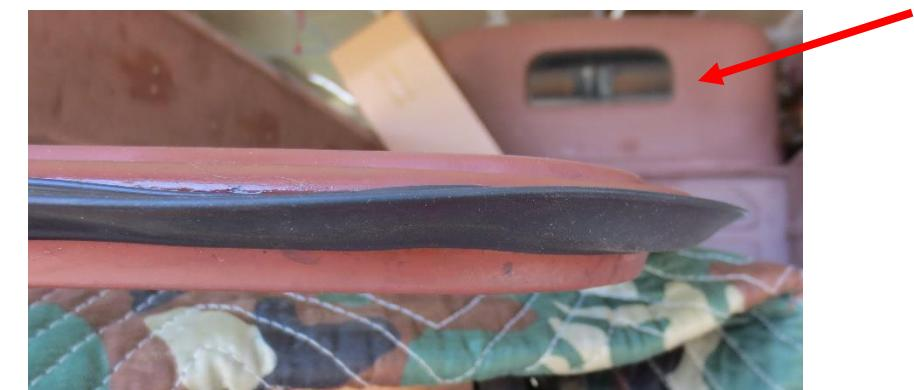
8. As you can see, this will straighten to gasket out for better sealing. RTV Silicone can be applied to hold the rubber in place.
