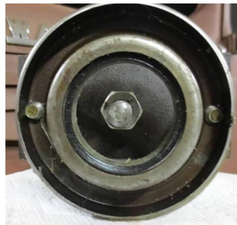
**Pinion Oil Seal Puller** – Another method is to weld a pipe to the seal and then wiggle it out.
