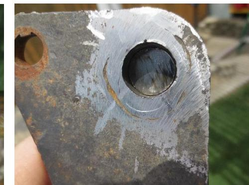
5. Next, check for straightness to the plate, and weld up.
