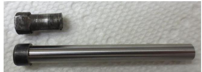
6. Using the  $\frac{1}{4}$  shaft determine the length from inside the housing wall and set screw hole and mark the pin using a permanent marker or other method. Cut the mark using a high-speed cut-off tool. Fit the pin in the pin hole to check the alignment of the notch to the set screw hole. Any adjustment should be cut towards the cutter end of the pin.
