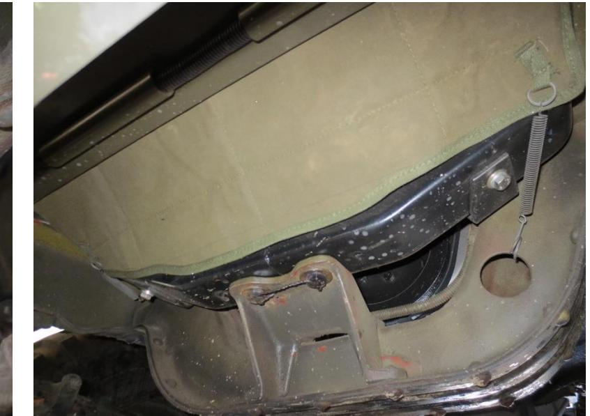
bb. **Installing the SS Fuel Tank on the M37 Truck.**
