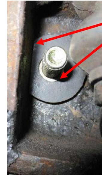
Make sure the insulator clears the side of the mount, and in the spacer. Tighten bolt/nut till tight. **Option** – Use a lock washer and nylon locking nut.
