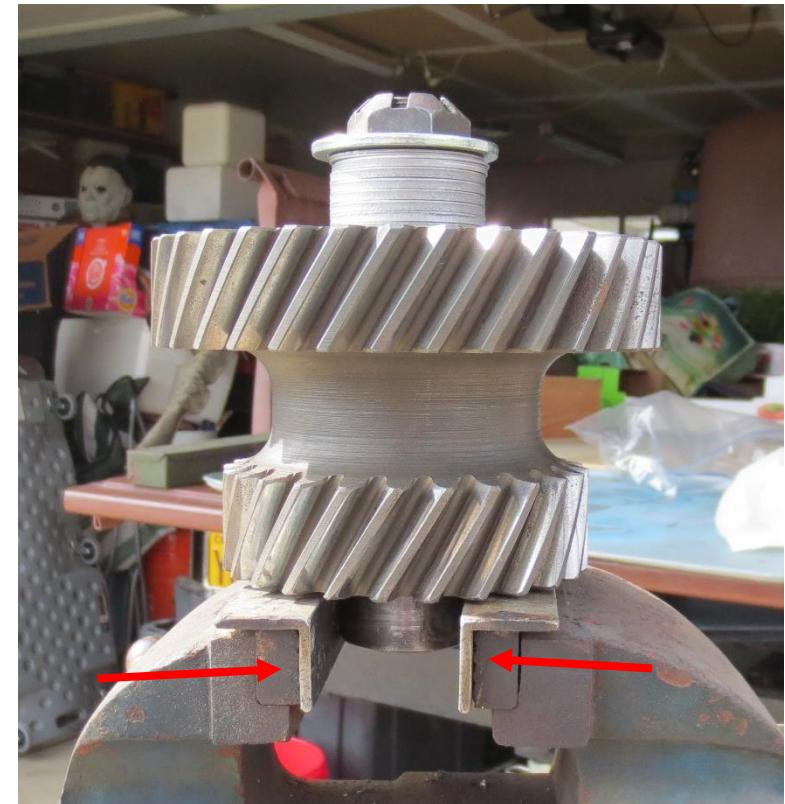
Once the bearings are adjusted, you are ready to install in the case. You can make a dummy shaft to hold the bearings, shims and spacer in place using 1-1/4 OD PVC pipe 3-15/16 long or you can buy a dummy shaft to use. Lube the shaft and housing holes to avoid friction build-up to allow the shaft to move easily when driven in using a brass drift and hammer. Drive enough to get the washer and nut on to finish pulling the shaft through, DO NOT PRESS through.
