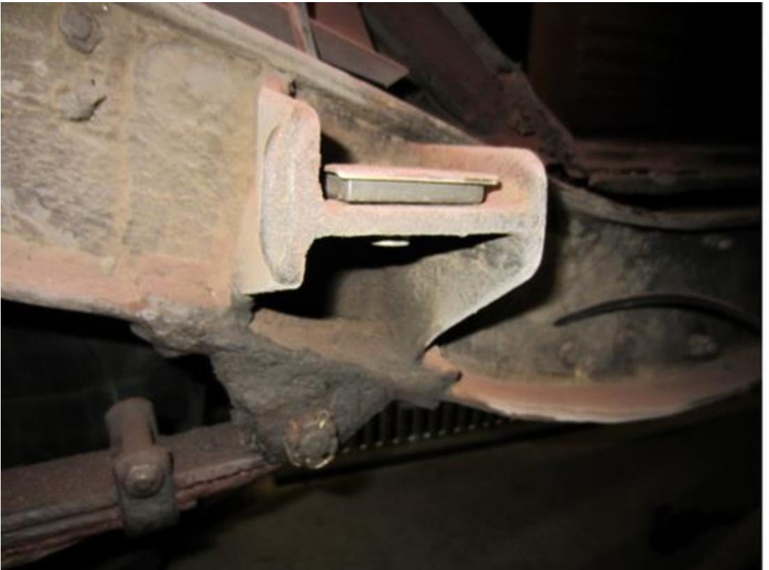
7. Images below show the insulators installed and the gaps between the PTO housing and the clutch fork lever.
