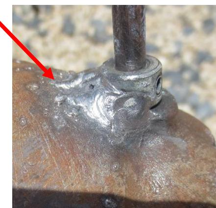
5. Measure the length from inside the housing wall to outside the collar and cut the new pin to length using a high-speed cut-off tool.
