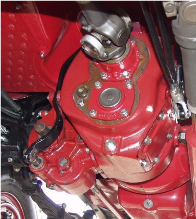
Fabricated bracket/lever to replace cable-controlled PTO.
