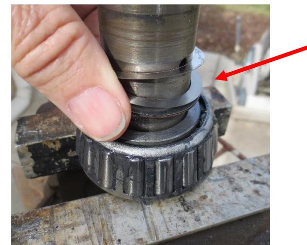
Assemble the shaft, bearings, spacer, shims, and nut, and place in a vice. Make sure you use soft metal to hold the shaft in the jaws. After you tighten the nut, open the vice jaws past the bearing cone and take a brass punch and hammer and seat the bearings by striking each end of the shaft.
