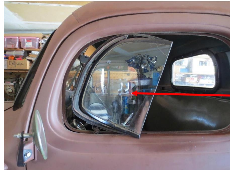
15. If after you install the ventilator, you may find that there is not enough clearance between the frame and weatherstrip at the points indicated, the frame is probably sprung by Auto Glass Technicians using tools to remove the glass in prior repairs. To correct, you will need to remove the glass from the frame while the frame is installed.
