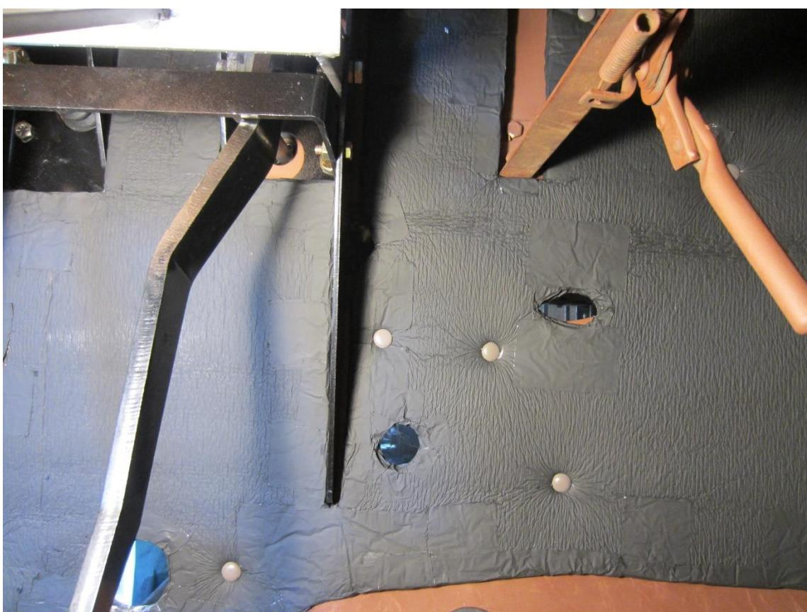
**You will need to modify the firewall insulating pad to work with the new mount. This one is made from insulating plastic foam, 2 layered, and painted flat black.**
