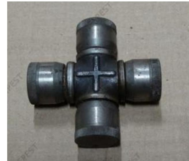
In order to identify a replacement part for Cleveland and Mechanics type journal assemblies, take the measurements of the cross section only, as shown in the illustration.
