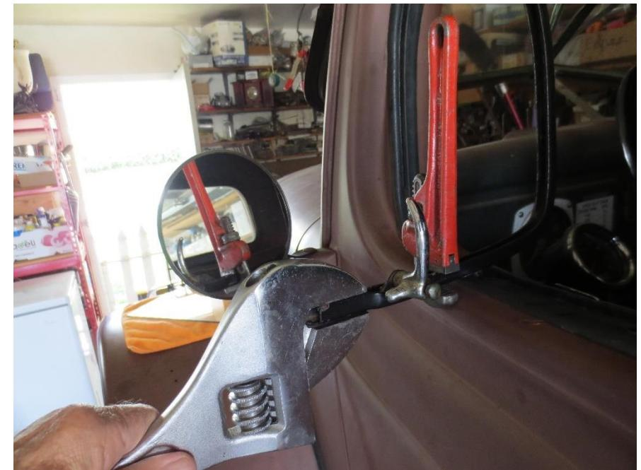
17. Repeat the process until the frame slides easily over the weatherstrip, then re-installed the glass.
