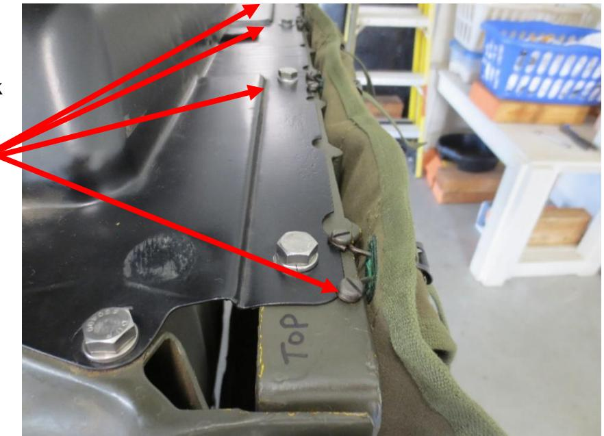
2. The next step is marking the side flat loops by placing the loop on the headlight guard, lining up the brass slot grommet with the loop and marking the holes. Remove the guard, mark drill points on the opposite side of the guard to facilitate drilling and taping. Install the brass grommets on the flat loops and lace the hold down straps. Complete both guards. The angled wire loops and sheet metal screws are not used.
