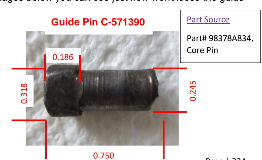
2. Grind the outer head off the pin and punch it out the housing.
