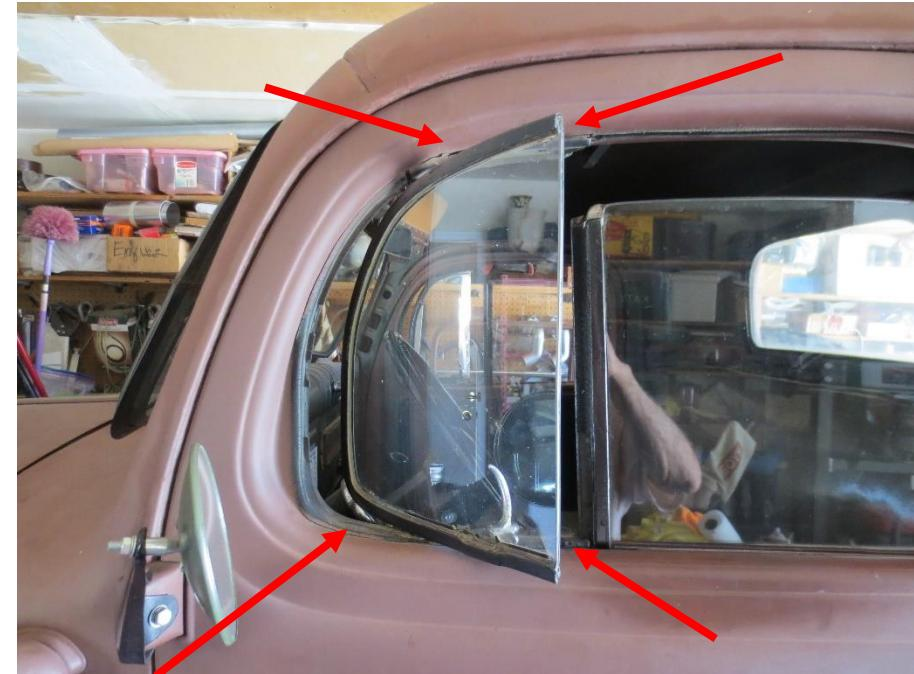
2. Once the screws are removed, roll the wing towards the rear of the truck. You may need to open the window to facilitate removing the wing and spring the frame some.
