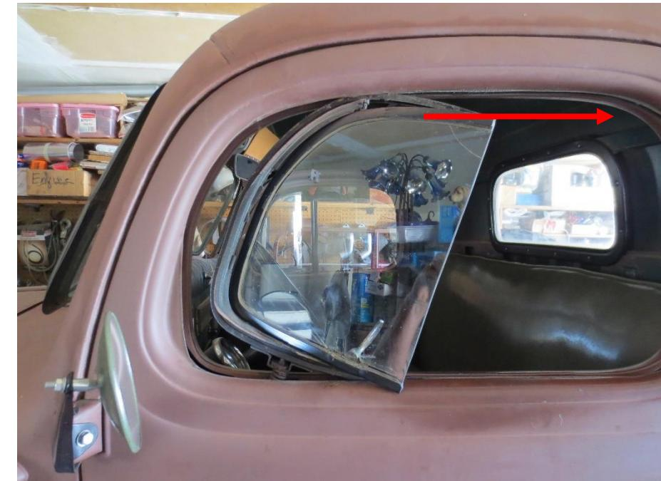
3. Next remove the screw and lock and back off the adjustment screw until the wing frame can be separated from the pivot adjustment screw.
