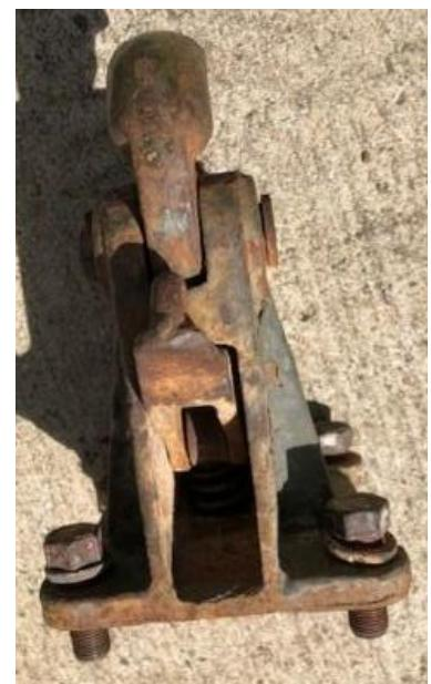
**Dodge M37 Cargo Truck, M42 Command Truck, M271/V41 Maintenance Truck (T-245 4x4) Pintle Hook Assembly [Stock No. G503-77073209, FSN 2540-707-3209, NSN 2540-00-835-9039, Holland Hitch Co. No. A86A10, CC-1268500]**
