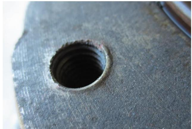
As you can see in this photo, light grinding, and chamfering was performed to correct the condition allowing the brake bracket to mesh with the retainer and seal properly.
