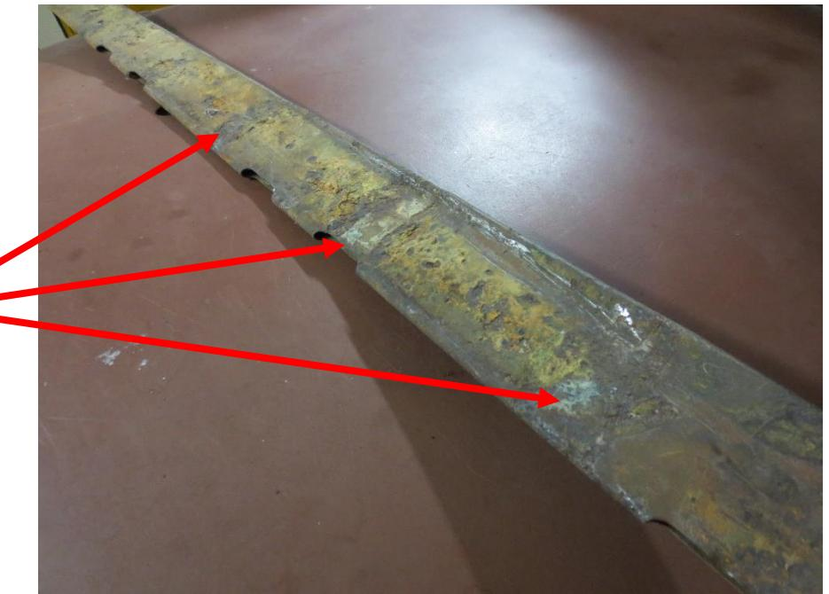
To loosen the tube from the block, use a 36" x  $\frac{1}{4}$ " rod, sharpen one end to a chisel point to tap along the tube on both sides to break it away from the block. You can see the score marks on the tube that was removed from an engine on the image below.
