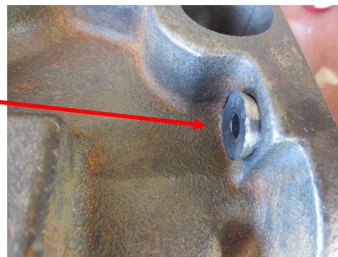
6. Next, mark the screw using a felt pin for a side grind.
