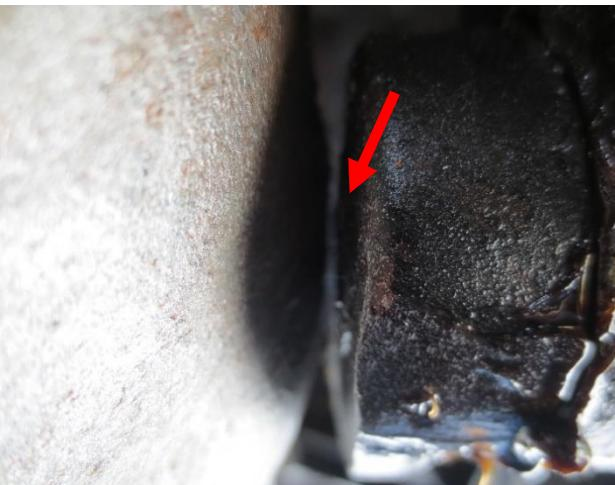
Clearance between the cab transmission cover and the top of the gearshift lever housing. If you cannot get a 1/16 wire between the housing and cab trans cover all the way around, you need to add rubber shims to raise the cab.
