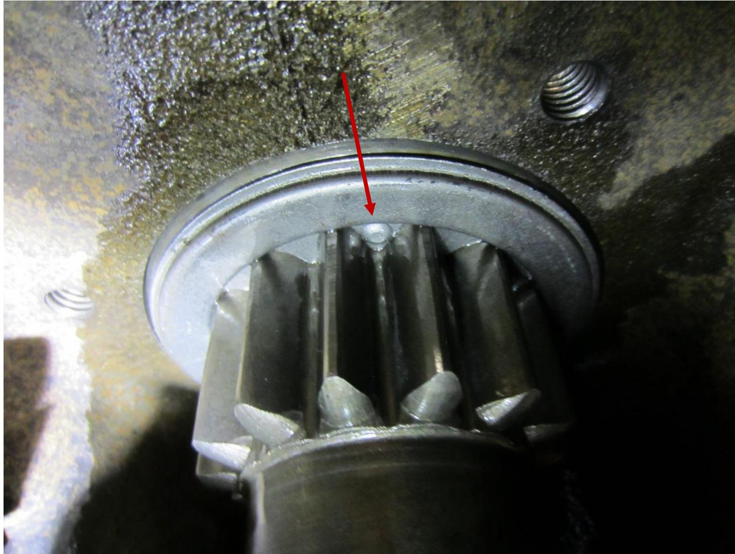
As far as the keys used on the first gear, both ends have a slight flare to them. If you file or grind one end to remove the flare, it will allow for easy use to align each gear when installing and final installation of the keys once all gears have been installed on the first gear.
