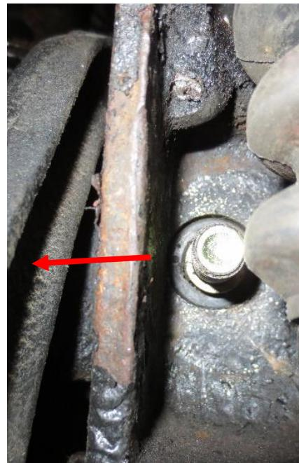
Remove the spacer and insulator from the side of the mount. You Will need to work it down between levers. Arrow indicates direction.
