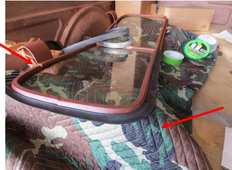
7. The gasket at the corners will tend to fold towards the front of the truck. This can be corrected by adding a piece of rubber under frame and gasket.
