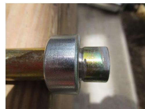
4. Next, you are ready to grind the end to the old shaft diameter. Be sure to keep the grinder parallel to the shaft for a straight grind. You can roll the shaft back and forth on a block of wood to facilitate grinding.
