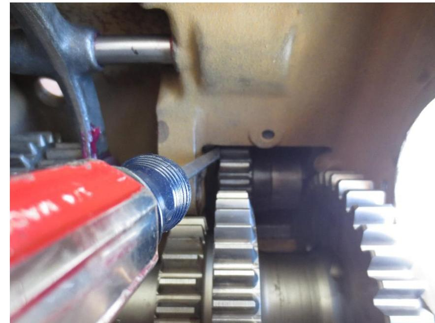
7. Using a dial indicator, rock the cluster gear back and forth to check backlash. Backlash should be set between .003 and .008. Once desired backlash is achieved, use gasket cement on gaskets and bolt threads when installing PTO.
