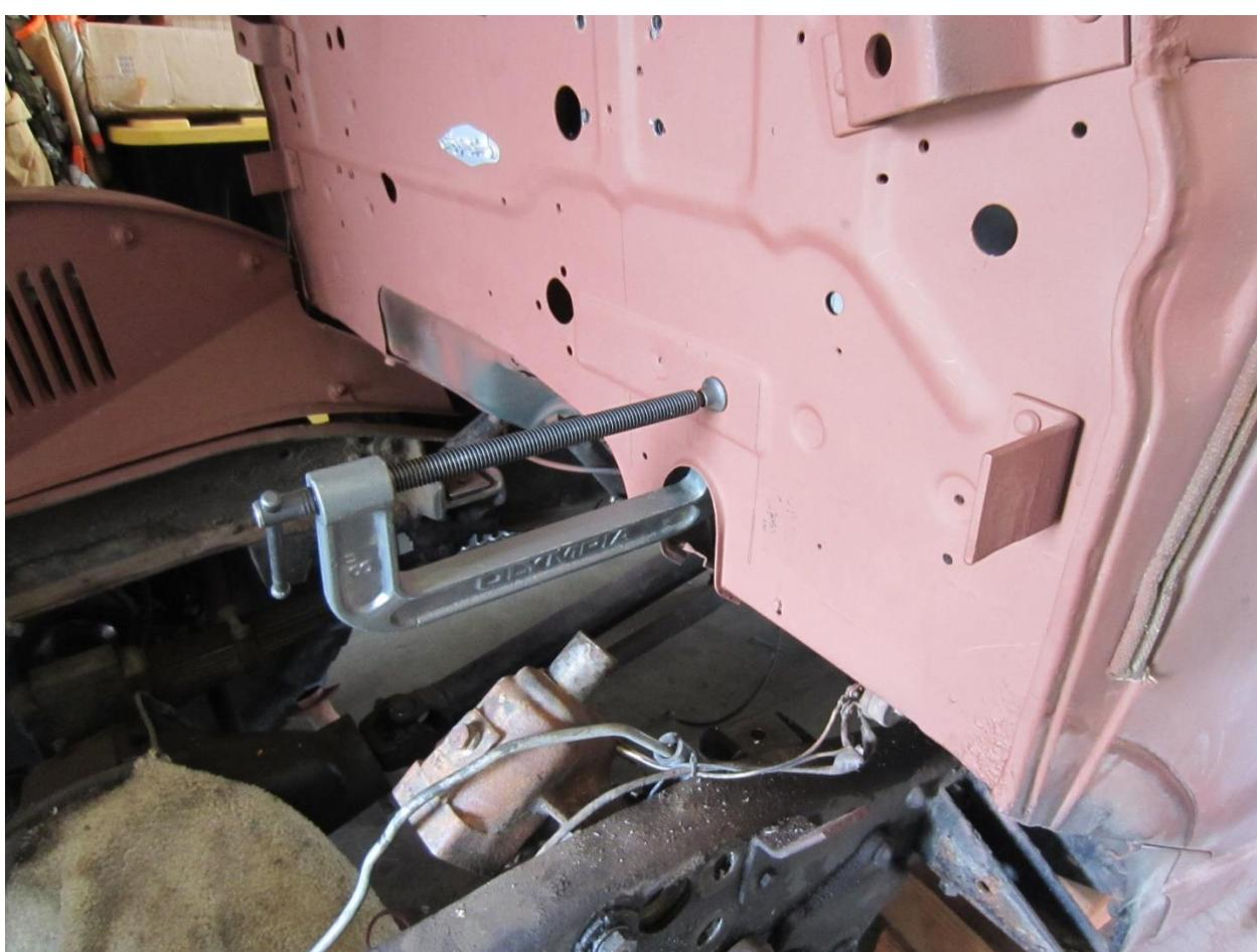
**It is recommended that a brace be made to prevent flexing of the cowl when pedals are pressed. This brace is home made and connects to the mount at a pressure point and connects the dash at the steering tube mount bolts. Tube mount/dash bolts were redrilled to  $\frac{1}{2}$  inch.**
