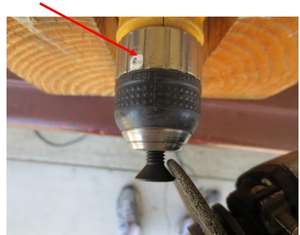
4. Periodically remove the screw and check the angle to see if any adjustment in grinding angle is required. You can use an angle finder for this purpose. Compare against the degrees as well as the side of the finder, line the screw up with the side of the finder.
