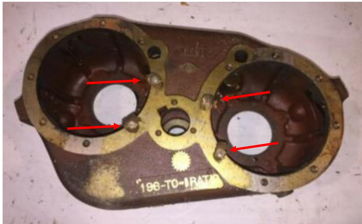
If changing the Ring & Pinion 5:83 ratio to 4:89 or installing larger tires, you will need to install a C-561816 Ring Gear in the TC so the speedometer will display the MPH more accurately. You can see from the image below, that it is difficult to determine which gear is 4 teeth or 5 teeth. The only way to know for sure is to read the part number on the side of the gear.
