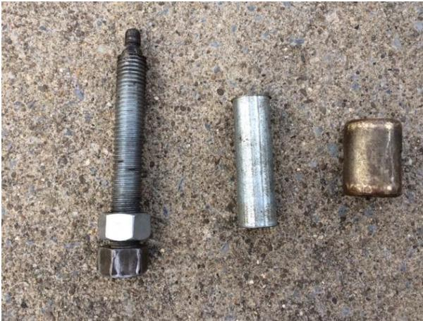
**Hub Puller** - Pulls front and rear hubs by switching the joint nuts/bolts to the opposite side.
