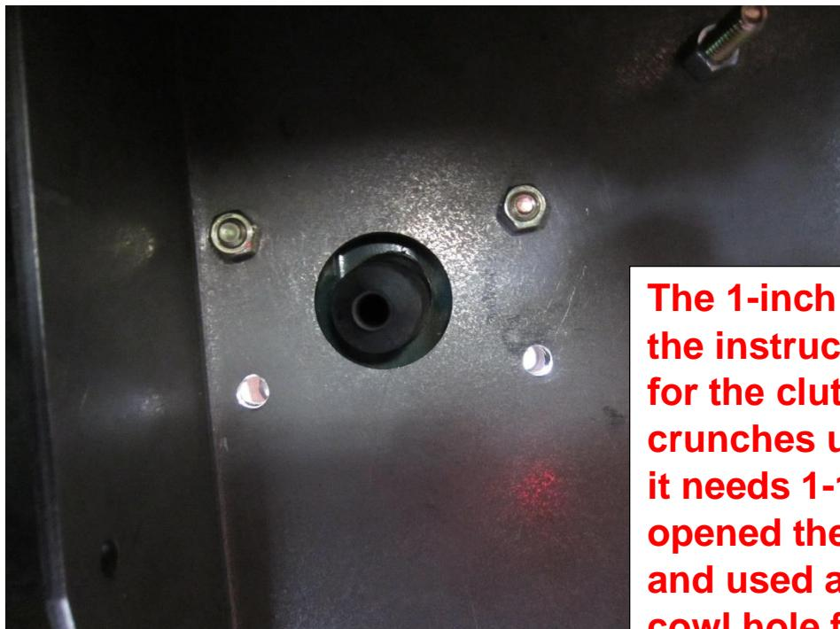
The 1-inch hole called for in the instructions is too tight for the clutch MC's boot, it crunches up against the cowl, it needs  $1\frac{1}{4}$  inch, so I opened the hole to  $1\frac{1}{2}$  inch and used a grommet in the cowl hole for the boot to rub against to avoid the boot tearing over time.
