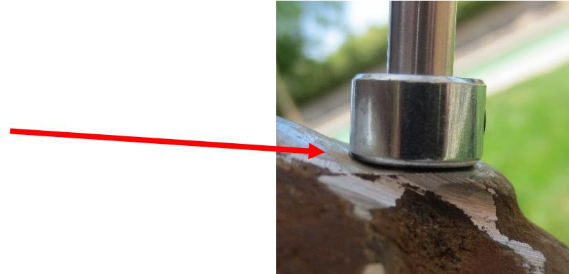
4. Align the collar using a  $\frac{1}{4}$  inch shaft and tack or weld the collar in place.
