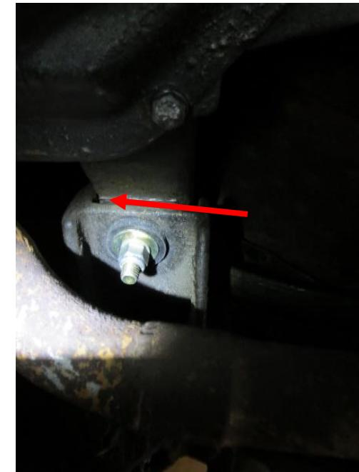
Remove the spacer and insulator from the side of the mount and up past the bell housing.
