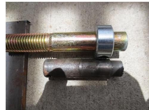
3. Using a cut-off tool or other tool, cut a groove around the shaft the depth of the old shaft.
