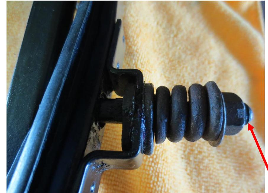
12. Next, seat the pivot adjustment screw and back off until the lock can be installed or  $\frac{1}{2}$  additional turn to give good clearance. Then install the lock and screw. You may want to use some anti-seize on screw threads.
